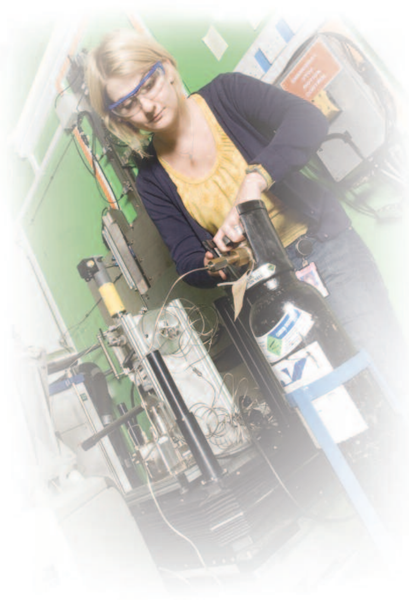
Instrument scientist Dr Sarah Rogers(ISIS), releasing CO 2 into a pressure cell at the sample position on the Sans2d instrument.
