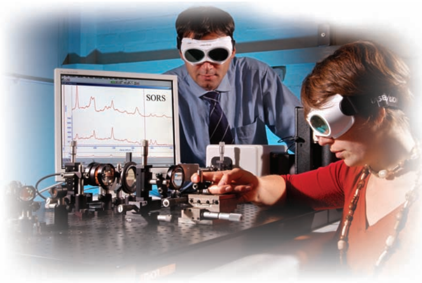
Aligning the Spatially Offset Raman Spectroscopy (SORS) instrument
