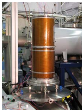
The new short path absorption cell with the outer vacuum jackets removed showing the copper strip heaters that will allow the cell to reach 470 K for high-pressure water vapour measurements as part of CAVIAR.
