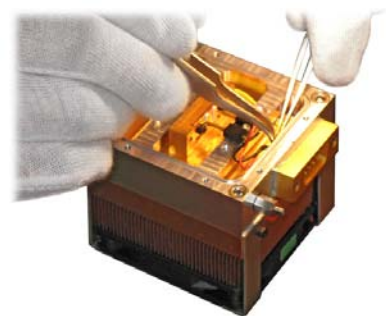
Quantum cascade laser systems are being developed through other activities at RAL. This benefits the MSF through the availability of state-of-the-art equipment such as this in-house room-temperature continuous-wave QC laser head.
