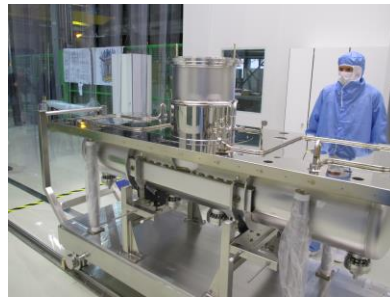
Progress - Graeme Barlow with the first cryomodule for HIE-ISOLDE. Every nut in this picture has been carefully cleaned. © CERN
