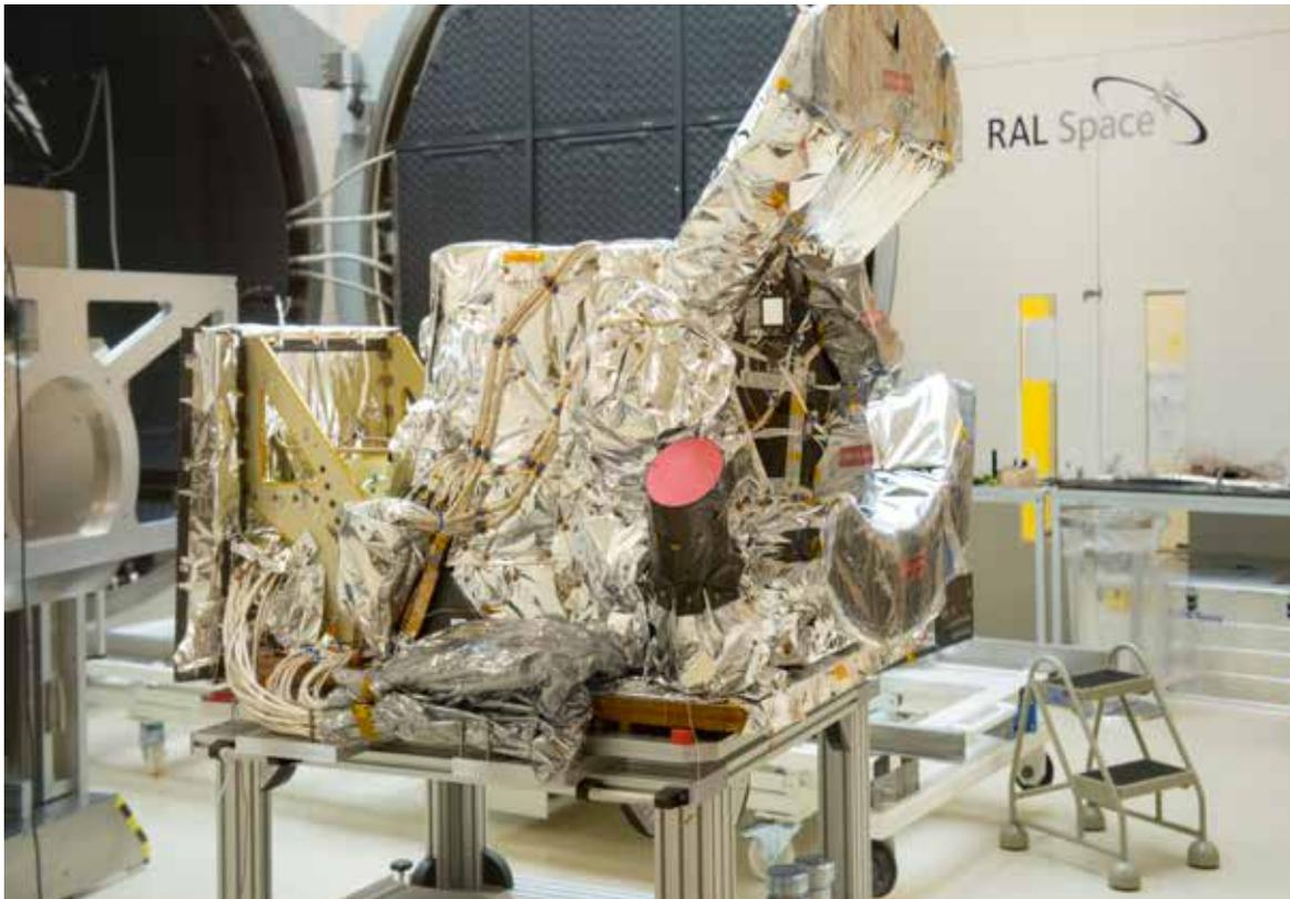
SLSTR undergoes calibration testing in the UKCCSI
