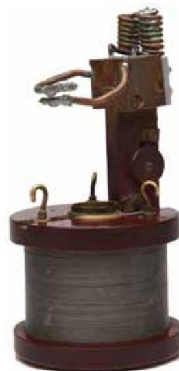
Figure 1, the first superconducting magnet manufactured by Oxford Instruments.
