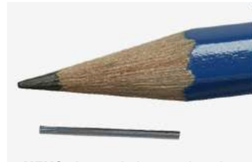
MEMS piezoresistive sensing element
