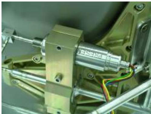
PRESENS sensor assembled to PRISMA spacecraft
