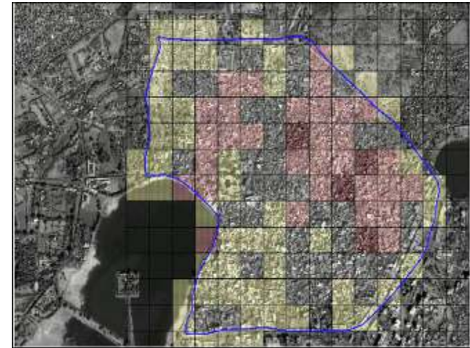
Building damage classification map of Bhuj, India
