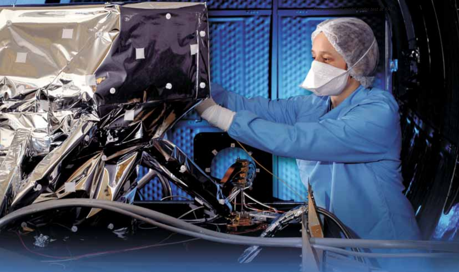
A member of the Thermal Engineering Group prepares a prototype of the Mid-Infrared Instrument (MIRI) of the James Webb Space Telescope (JWST) for cryogenic testing in SSTD's Space Test Chamber
