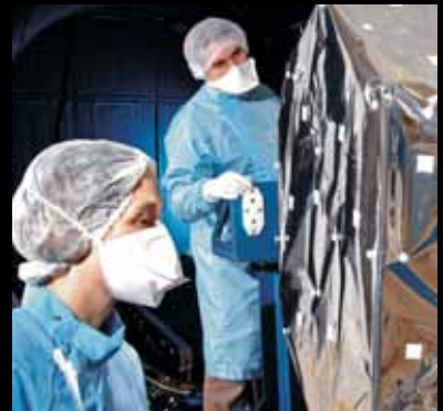
Thermal model of the JWST MIRI instrument MLI (inset) and photo-type MLI blankets during preparation for thermal balance testing
