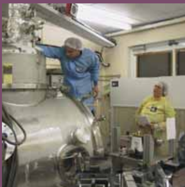
1.7 K test cryostat for the Herschel/SPIRE instrument. Thermal design, analysis and verification of the instrument was carried out at RAL
